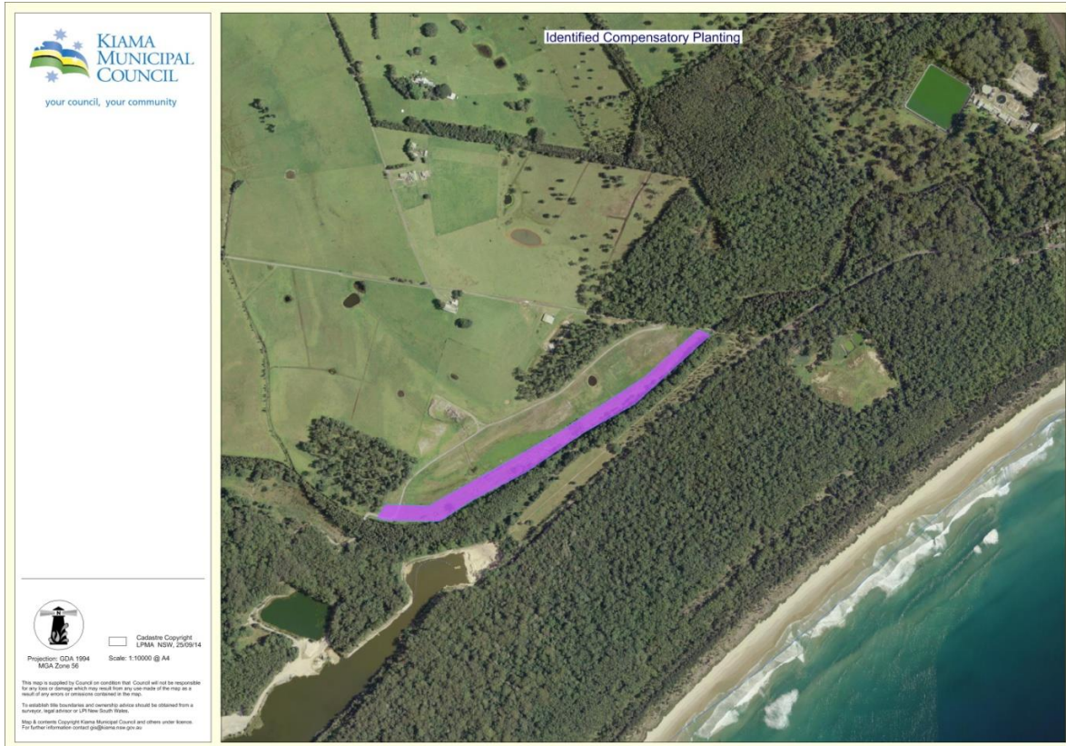
Figure 24: Future compensatory planting for Blue Angle Creek which will reduce the potential for flood scour
