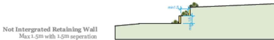
Figure 28: Non-integrated retaining wall (greater than 1.5m) (DKO, 2023)
