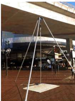
6m high free standing tripod aerial rig
