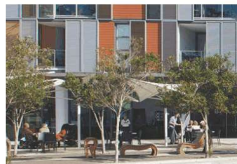
Generous floor to ceiling heights are particularly important for ground floors to be able to accommodate change of uses over time and maintain a positive relationship with the street
