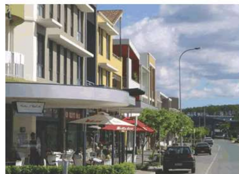
Example of buildings along a built-to alignment, which helps define the street edge and create direct connections between ground floors and the footpath
